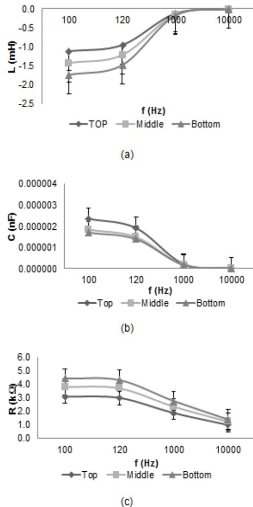
Figure 2. Bioelectrical Properties of Sugarcane at various frequencies: (a) Inductance (L), Capacitance (C) and Resistance (C)
